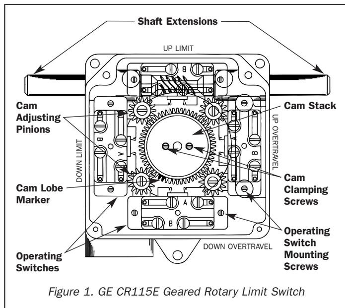
Figure 1. GE CR115E Geared Rotary Limit Switch
